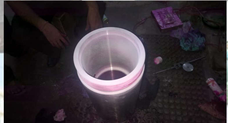
Visible Dye Penetrant Testing of Forged/Machined item
